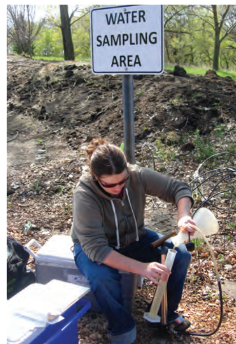
Water samples were analyzed for 18 constituents, including pH, nitrate-nitrites, phosphorus, potassium, the standard EPA Part 503 metals panel, silver, copper, mercury, nickel, zinc and TKN.
