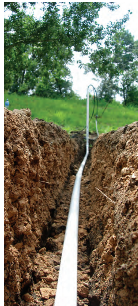
The lysimeters were buried at a depth of 36 inches and placed under negative pressure to allow for collection of contact water that infiltrated into the subsoils.
